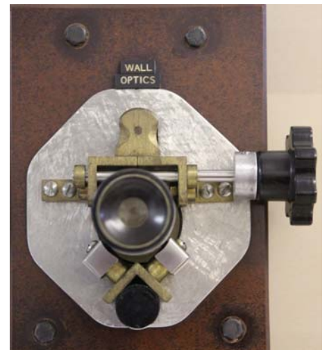
The original Crayford eyepiece mount, now in the possession of the Crayford Manor House Astronomical Society. Photo by Mike Rushton.
